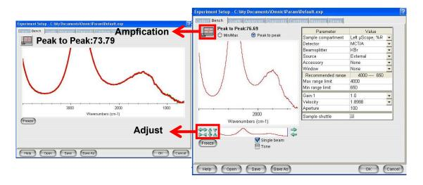
When clicking the measurement button, the spectrum displayed in green will remain fixed, representing the signal under the current focus. This serves as a reference for focusing adjustment. Normally, a clear signal will appear when the sample is in focus. Adjust the focal position to the point where the signal is strongest.
