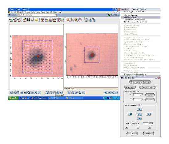
Once the parameters (e.g., scan count, step size) and sample position are set, go to the Collect window, select Collect Map, assign a file name, and start scanning the sample.
